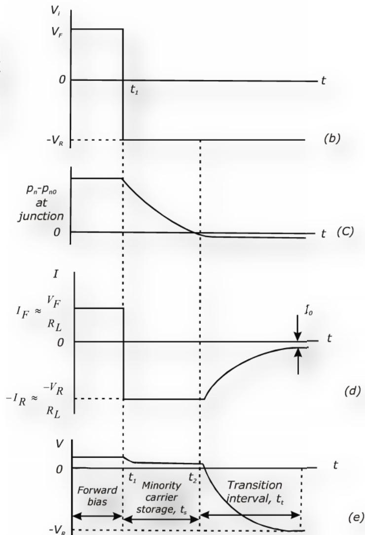
Fig 2: Storage & Transition Times during the Diode Switching
