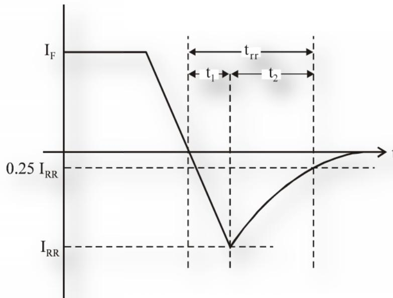
Fig 3 Reverse Recovery Characteristics
