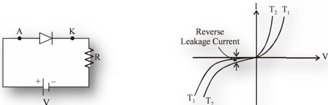
Fig 1 Diode Characteristics
