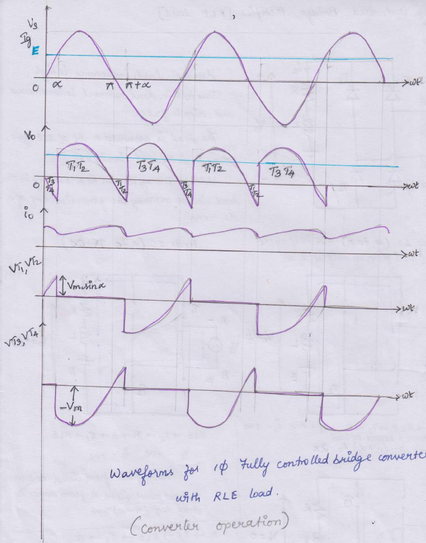
Waveforms for 1φ Fully controlled bridge converter
