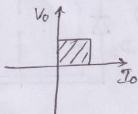
1φ Half controlled bridge rectifier with R load
