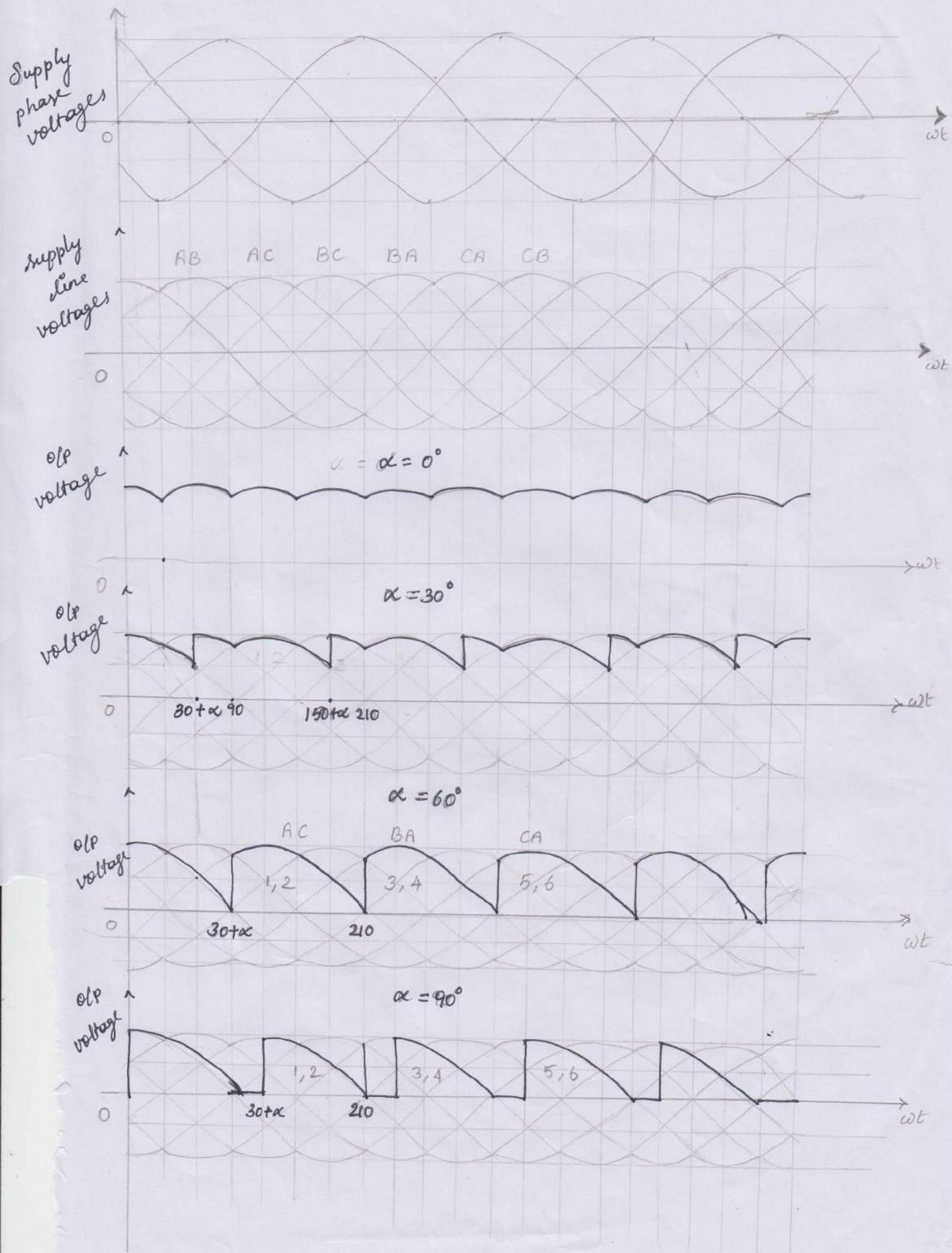
3φ Half controlled converter with, RL Load.
