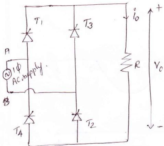
1Φ Fully controlled bridge rectifier consists of 4 SCR's.
