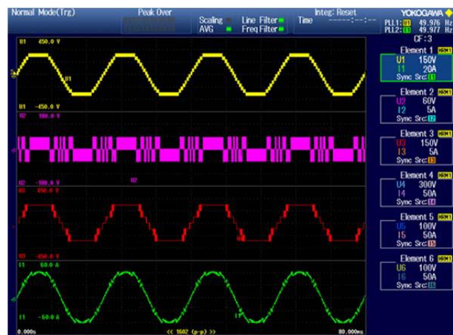
Fig. 22. Hardware results with capacitor voltage balancing algorithm (a) Voltage across the load (15 Levels) (b) Voltage across the HSFI V_{up} (c) Voltage across the LSFI V_{low} (d) Load Current waveform for modulation index M_a=1 .
