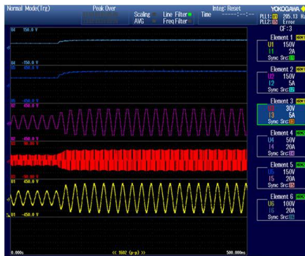
Fig. 19. Step response in capacitor voltages of HSFI and LSFI along with HSFI, LSFI and load voltage waveform.
