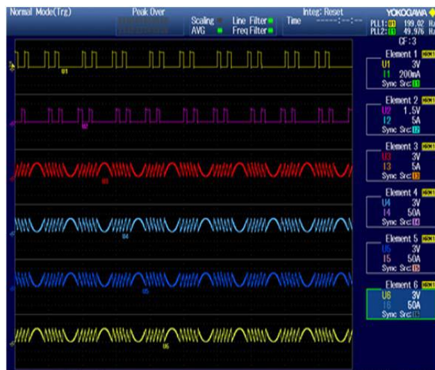
Fig. 20. Switching pulses and reference waveforms (a) Auxiliary switch 1 (b) Auxiliary switch 2 (c, d, e and f) Reference waveforms of the HSFI [Without capacitor voltage balancing].
