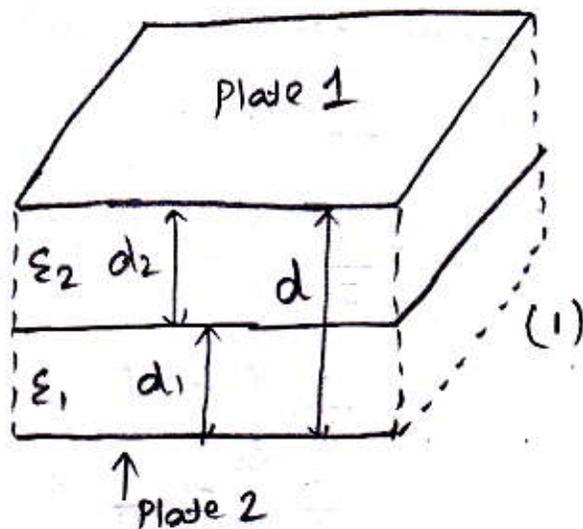
$$V = V_1 + V_2 = E_1 d_1 + E_2 d_2 \quad \text{--- (1)} \quad (4)$$
