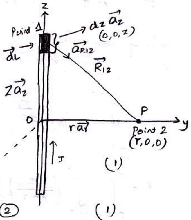
Thus total Flux intensity  $\vec{H}$  can be obtained by integrating  $d\vec{H}$  over the entire length of the conductor
