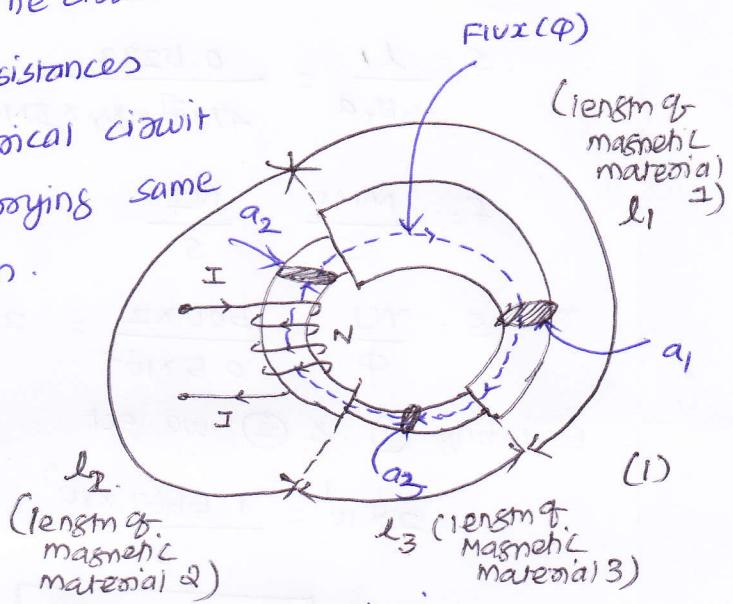
The total resistance of the electric circuit is  $R_1 + R_2 + R_3$ . May the total reluctance of the magnetic circuit
