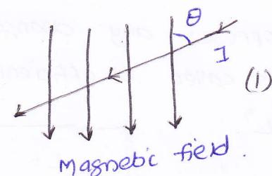
As shown in figure below, if conductor is kept along the lines of magnetic field then  $\theta = 0^\circ$  and as  $\sin 0^\circ = 0$ , the force experienced by the conductor is also zero.
