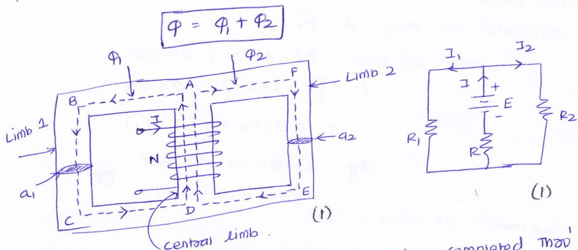
The fluxes  $\Phi_1$  and  $\Phi_2$  have their paths completed through ABCD and AFED respectively. This is analogous to division of current in case of parallel connection of two resistances in an electric circuit as shown in figure above.
