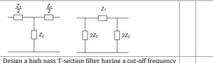
Design a high pass T-section filter having a cut-off frequency of 1000Hz to operate with a terminated load resistance of 600Ω.
