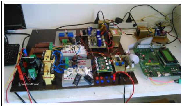
Figure 17. Laboratory Prototype of the proposed PV fed Single stage boost Inverter.
