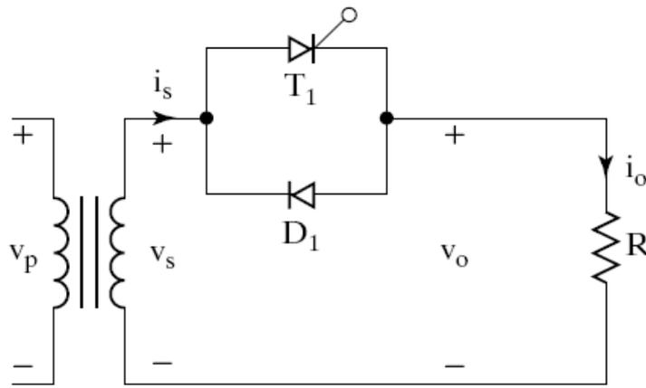
**Fig.: Halfwave AC phase controller (Unidirectional Controller)**
