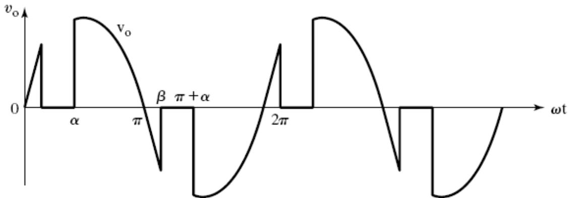
When  $\alpha > \phi$ , the load current and load voltage waveforms become discontinuous as shown in the figure above.
