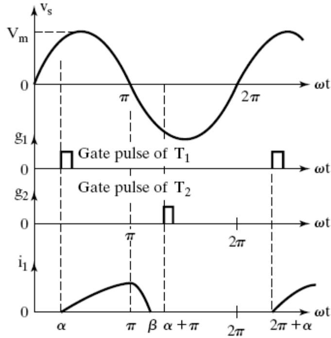
**Fig.: Input supply voltage & Thyristor current waveforms**
