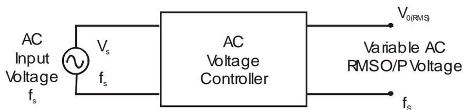
There are two different types of thyristor control used in practice to control the ac power flow
