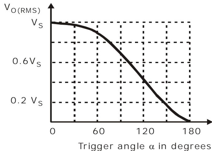
We can notice from the figure, that we obtain a much better output control characteristic by using a single phase full wave ac voltage controller. The RMS output voltage can be varied from a maximum of 100%  $V_s$  at  $\alpha = 0$  to a minimum of '0' at  $\alpha = 180^\circ$ . Thus we get a full range output voltage control by using a single phase full wave ac voltage controller.
