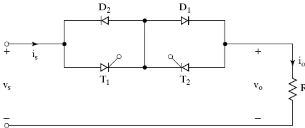
**Fig.: Single phase full wave ac controller with common cathode (Bidirectional controller in common cathode configuration)**
