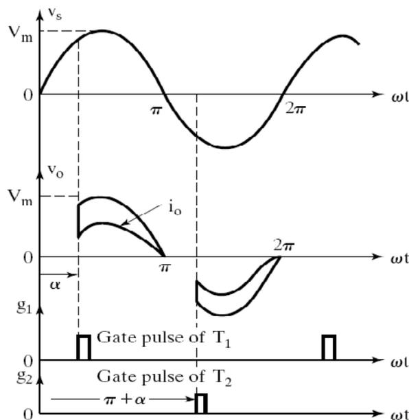
**Fig: Waveforms of single phase full wave ac voltage controller**
