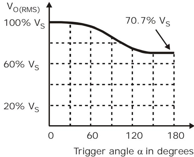
**Fig.: Control characteristics of single phase half-wave phase controlled ac voltage controller**
